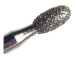
C. The tungsten carbide engraver is very useful for breaking extremely hard encrustations. However, it is very very sharp, and if your hand slips you can puncture and/or scratch the living daylights out of your finger, or worse, the coin (the finger will heal). It is also very useful for gently cleaning ridiculously tiny crevices, but you have to have a very very very steady hand, otherwise you will scratch the coin very very very easily.
