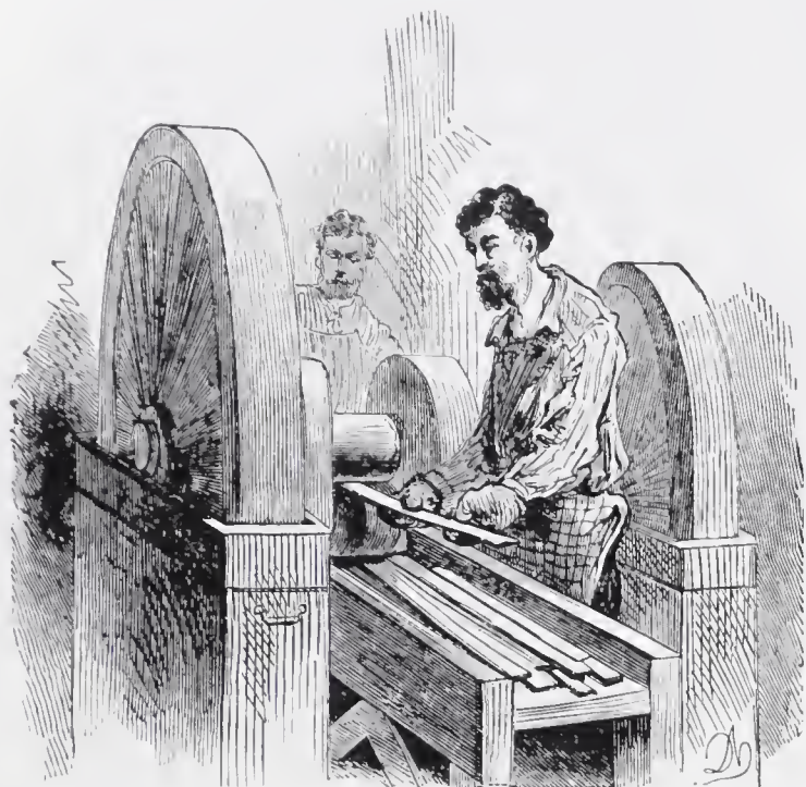
Rolling machine for the preparation of planchet strips.
