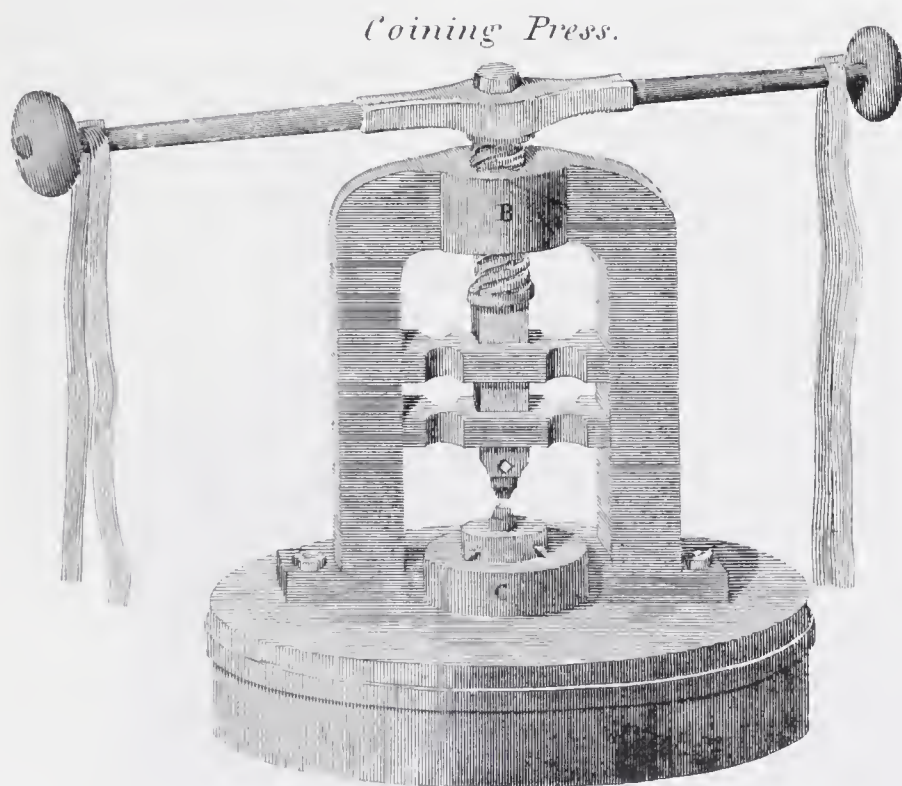
Early coining press of the general type used at the first Philadelphia Mint beginning in 1792. Operation was by hand.
